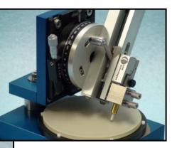
Radian<sup>™</sup> and Trig LT<sup>™</sup>'s precision rotary stages can be continuously adjusted to form a wide range of fiber tip angles.
