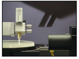
Trig LT<sup>™</sup> provides a video inspection module to offer realtime monitoring of the fiber during the polishing process.
